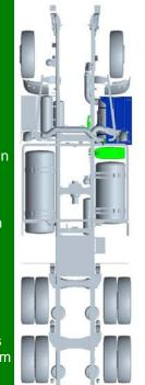
The SCR system components are integrated with the vehicle chassis. Vehicle packaging for these components is dependent upon exhaust configurations specified and the application. For example, in a typical vehicle, the DPF and SCR catalysts will most likely be positioned within the toolbox mounted under the cab as illustrated in blue in the rendering at left.
