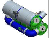
The DEF tank, noted in green in the rendering at left, will be mounted on the chassis in front of the fuel tanks in most configurations where refilling is simple and there is no interference with aftermarket-related modifications that occur behind the cab and/or sleeper.
